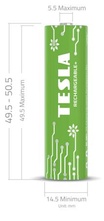
**DESCRIPTION:** Nickel Metal Hydride Rechargeable Battery, AA Size **CHEMICAL SYSTEM:** Nickel Metal Hydride SHELF LIFE: Guaranteed for 500 recharges **NOMINAL VOLTAGE:** 1,2 Volts NOMINAL DIMENSIONS: Ø 14,5 mm x 50,5 mm **TERMINALS:** Protruded positive(+) and flat negative (-) contacts JACKET: Foil jacket **APPLICATIONS:** All electronics devices e.g. toys, photographic equipment, audio appliances, lighting & torches. **STORAGE TEMPERATURE:** -20 ℃ to + 35 ℃ **NOMINAL WEIGHT:** 29 g
