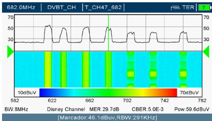
*Effect of a fading whereby the three high channels suffer variations in their signal level.*
