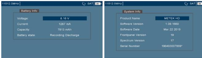
System adjustments screen / Battery and system information
