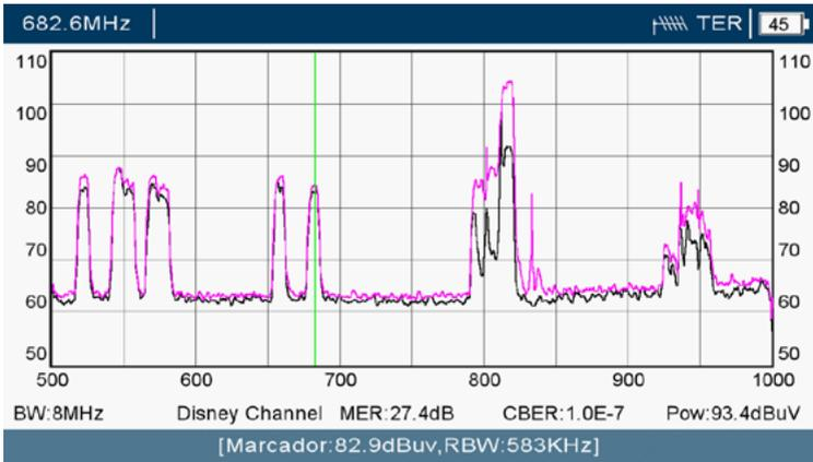
Image with seven TDT muxes and the maximum peaks of 3G/4G mobile telephony.
