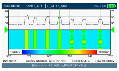
Effect of a fading whereby the three high channels suffer variations in their signal level.
