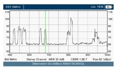
Measurement at the head including 3G and 4G signals (The downlink channels are observed at DVB-T channels)
