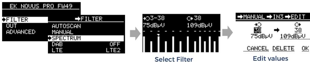
The SPECTRUM option allows you to perform the same actions on the filters as the MANUAL option, with the additional advantage that, at a glance, you can see all the programmed filters and there's no need to select the input. It is simply a powerful alternative, offering the installer the flexibility to choose the option they prefer for managing the filters according to their needs.
